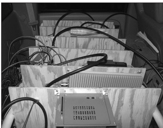
Figure 6 — K5GJ/r transverter mounting.
